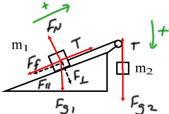
$$\begin{aligned}m_1 &= 2.0 \text{ kg} \\m_2 &= 3.0 \text{ kg} \\\theta &= 30.0^\circ \\\mu &= 0.15\end{aligned}$$
