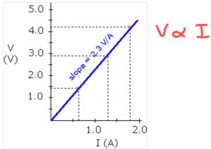
Note that V vs. I is a straight line which means that for this particular circuit element the ratio of potential difference to the current is constant. This **ratio** (which can be found by calculating the slope) is referred to as the **resistance**. The **slope** or **resistance** of this element is 2.3 V/A or 2.3  $\Omega$ .
