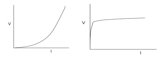
This graph is typical of a light bulb. Resistance increases as the filament heats up. This graph is typical of a diode, a semiconductor. Under lower voltages it behaves very much like an insulator. Then, when the voltage is right it "cuts in" and acts conductor!
