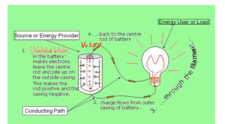
For the electrons, the casing is at a higher potential than the rod. Therefore if a path is provided, the electrons will run "downhill" to the top of the rod. (Later you will learn more about the potential energy **gain** in the battery and the potential energy **loss** in the lamp.)
