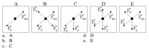
3. An object sits at rest on a ramp. Which of the following free-body diagrams best represents the forces acting on the object?
