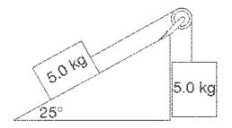
24. Two masses are connected with a rope that passes through a pulley. The coefficient of friction between the objects and the surface is 0.60. Assume that there is no friction in the pulley.
